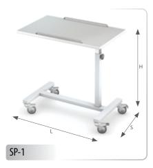
top of laminated chipboard frame of powder coated steel base of steel, equipped with 75 mm diameter castors, including two with lock option: frame and base of stainless steel grade 0H18N9 (AISI 304)
